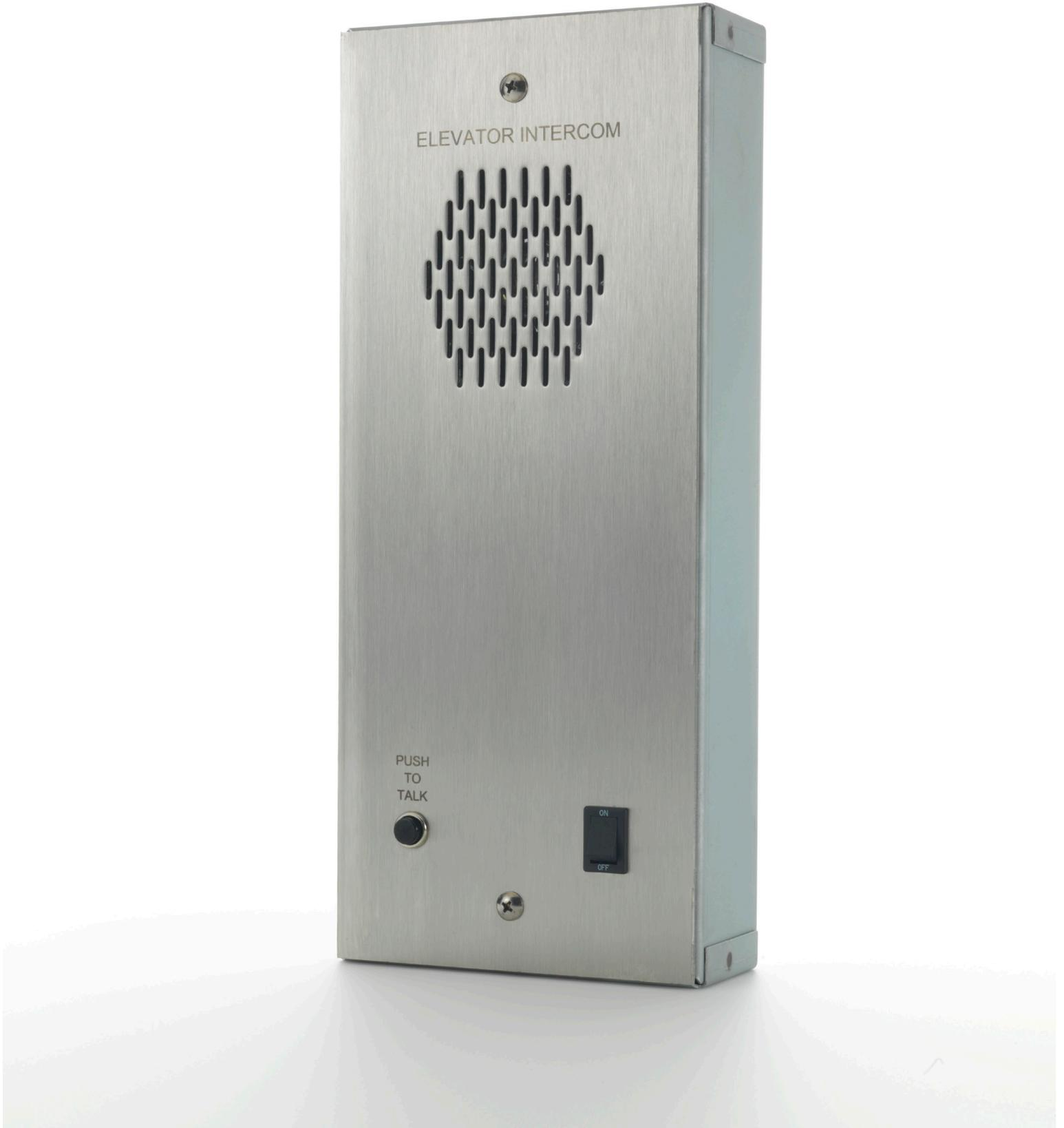
Everclear® intercom – Single car master station with #4 brushed stainless face plate and corrosion resistant EG steel enclosures for machine room surface mounting. Size 5-1/8" x 12-1/8" x 1-15/16" deep.
