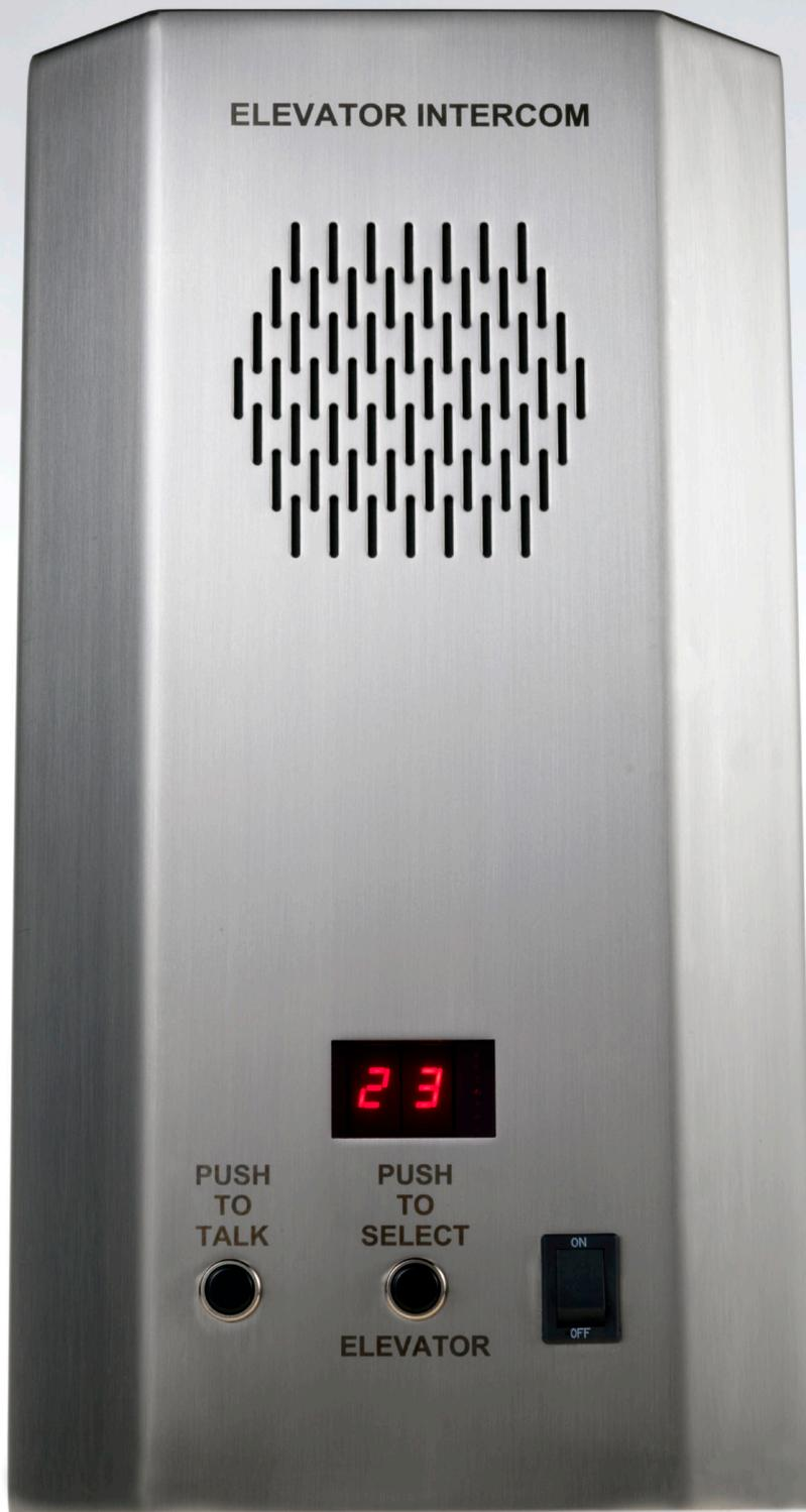
Everclear® intercom optional surface mounted lobby fixture with #4 brushed stainless finish, concealed fasteners, low-profile vandal resistant controls, 7-segment LED display (optional 2-digit display shown) and leveling slots for mounting. Size 6" x 12" x 1-3/4" deep. Multicar shown.
