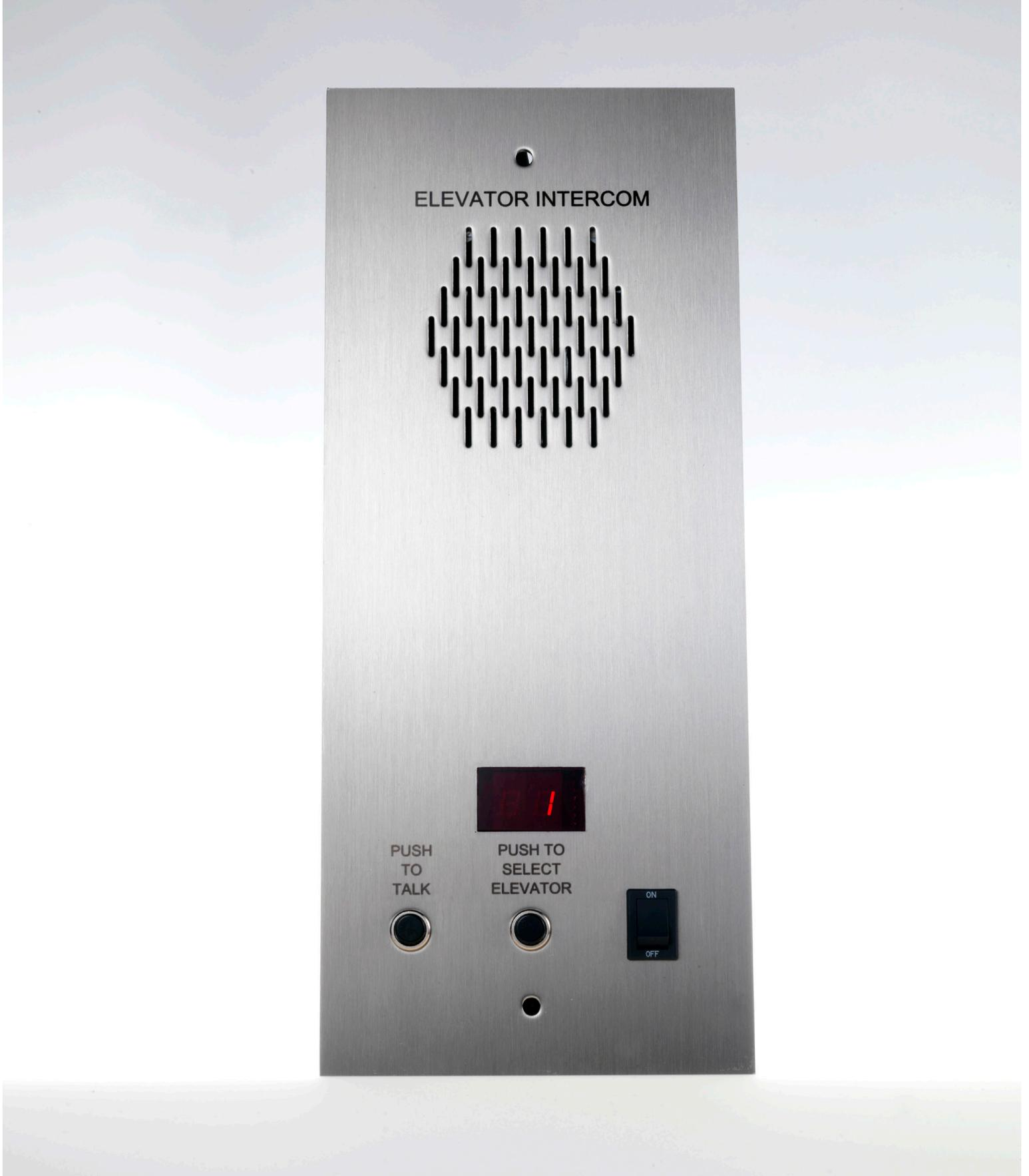
Everclear® intercom with #4 brushed stainless finish, low-profile vandal resistant controls and 7-segment LED display. Size 5" x 12". Standard EG steel corrosion resistant enclosures are flush mount (recessed) for lobby and surface mount for machine rooms (Multicar shown)
