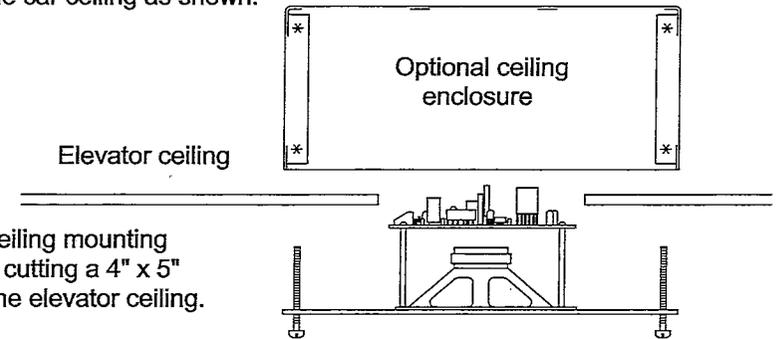
Above ceiling mounting requires cutting a 4" x 5" hole in the elevator ceiling.
